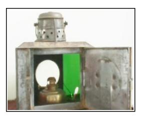
Ship's port/starboard combination bow lantern, late 1800's to early 1900's. It has two glass panels, one red, one green, and a brass kerosene tank with wick inside the lantern. It was donated by John and Becky Burnham. It has been in their Manset home for generations.
